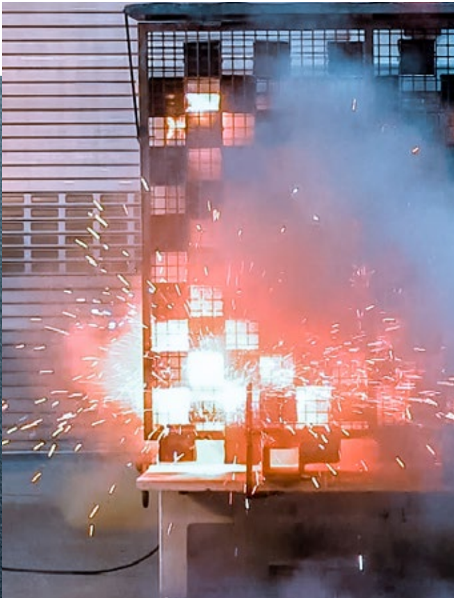
An arc short circuit resistance test according to IAC-A (20 kA / 1s)
