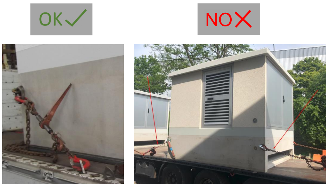
Fig. 10: Sling points on the outer face of longitudinal walls
