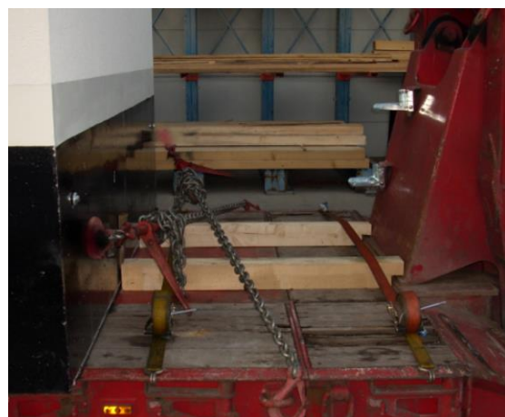
Fig. 16 Blocking with wedges or prisms
