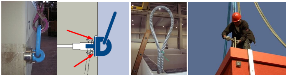
Fig. 21: Examples of correctly screwed lifting accessories
